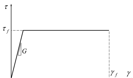
Figure 5. Ideal elastic–plastic shear model for the matrix material used in the plasticity analysis.
